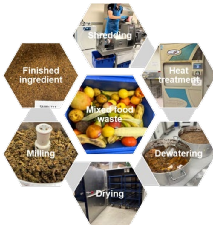
Figure 1: Process of treating mixed food waste into a dry feed ingredient. The material was initially macerated/shredded and then heat treated, dewatered, dried and milled into a feed ingredient.
