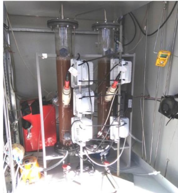
Figure 3 Schematic of the bubble reactor columns (left), photo of the reactors with PPB growing in the columns (right).
