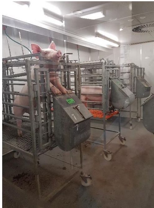
Figure 6. Overview of placement of the metabolic cages in the TN room are seen. Each metabolic cage has an individual water hose attached to supply water to the nipple drinkers. The food receptacles are assembled on the front end, which is also the opening to the cage. Pigs are pushed backwards into the cage and walk forwards when required to exit the cage.
