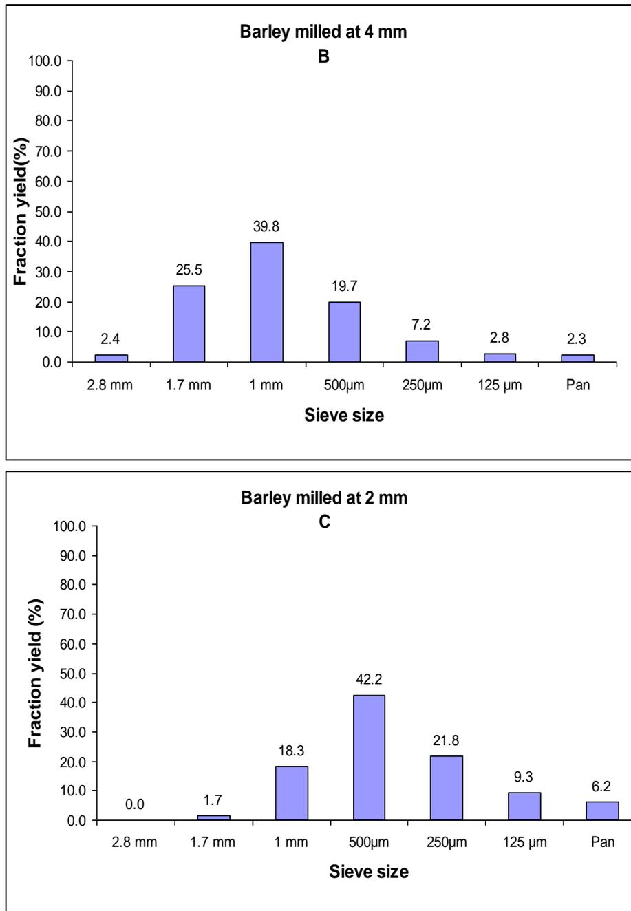
Figure 2 - Sieving analysis of barley milled through a 4 mm or 2mm screen.
