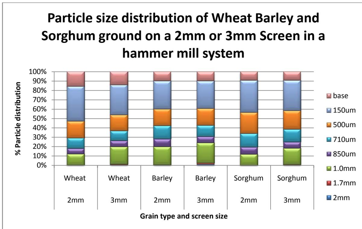
Figure 1. Particle Size distribution of wheat, barley and sorghum ground through a two and three millimetre screen in a hammer mill system.
